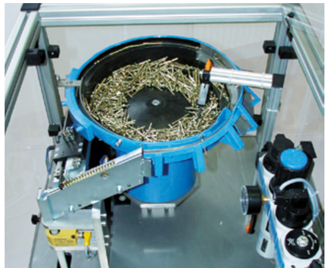
Fasteners are transferred from the bowl feeder to the placing head via the blow feeder
